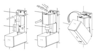
Reassembly the mechanism, the soap tank with the valve and the soap tank locator Close the unit
