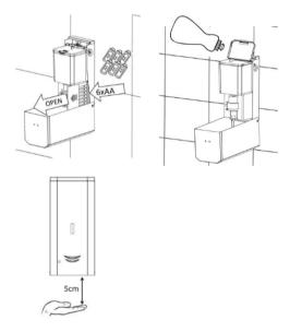
Open the unit with the provided key Remove the battery cover and install 6 Alkaline 1.5V AA batteries. The LED
